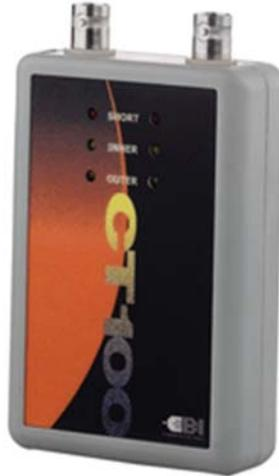
The CT100 Coaxial Cable Tester is a hand-held battery-powered unit for testing coaxial cable assemblies. It is suitable for "thin net" applications as well as CATV and RF/Microwave broadcast. Apart from indicating the usual "inner conductor open circuit," "outer conductor open circuit" and "short circuit" faults, the CT100 will indicate at which end the fault is situated.
