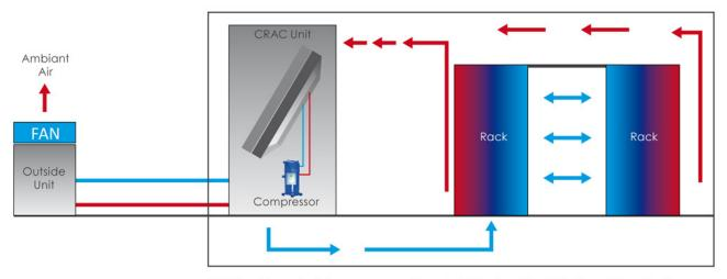
CRAC unit is cooled via compressor. There is DX-Mode , Mixed-Mode and Free Cooling Mode operation options
