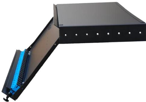
Linxcom designs and manufactures a unique and robust 19" 1U sliding patch panels. The patch panel consists of a few key elements: a universal chassis, adaptable to various applications; removable front frames, making changing the adapter type, loading or recessing adapters very easy; adjustable brackets, for fully recessing the whole panel for a better bend radius. Can hold up to 48 fibres housed within a 1U space.
